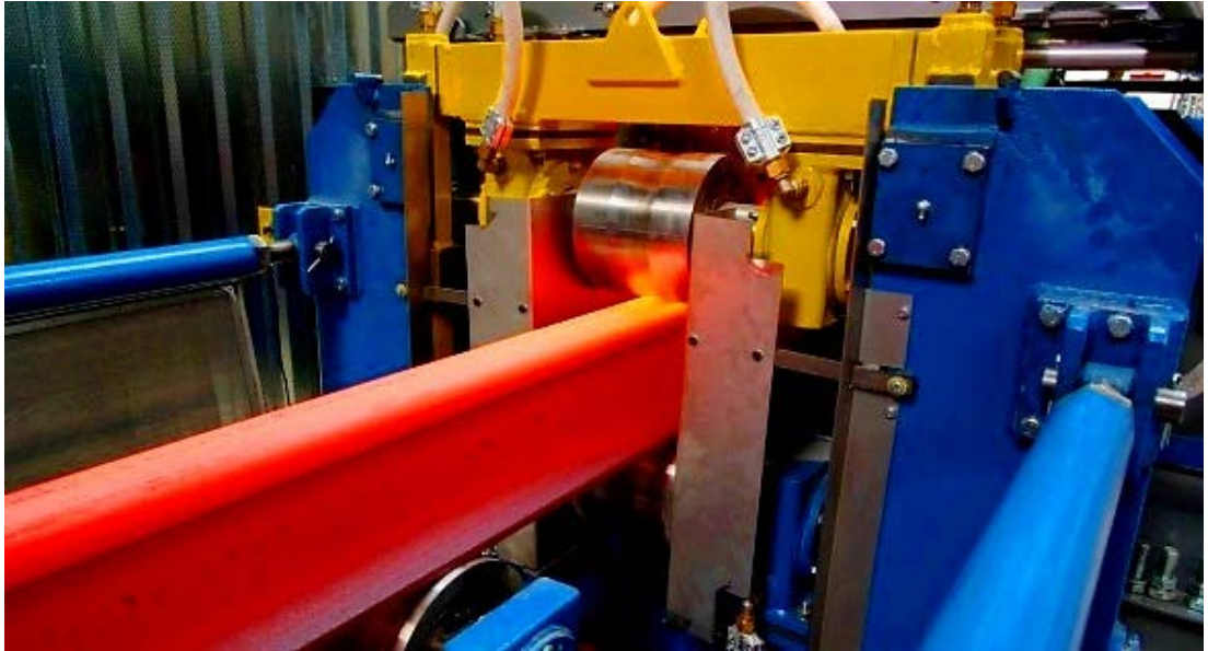
Rolling of Rail; British Steel
