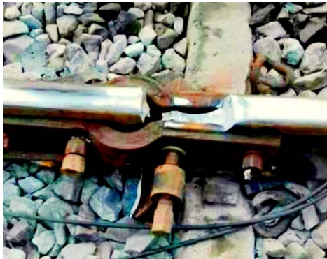
In-Service Rail- and Weld Failure; Central Railway, near Kalyan (left), near Badlapur (right)
