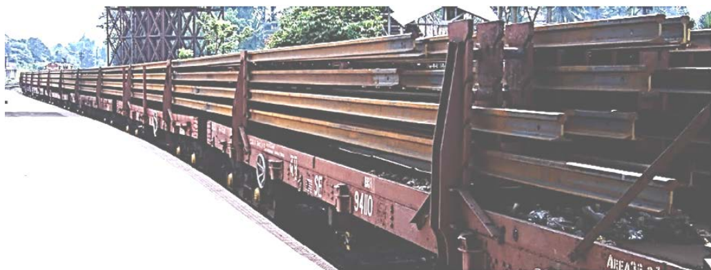
Rail Trailer with long rolled stationary Flash-Butt welded Bhilai, SAIL, Rail Panels (Londa, India); pict. by F. Wingler
