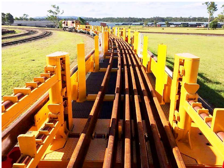
Robel Long Rail Transport Trailer, up to 500 m length
