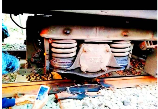
In-Service Rail- and Weld Failure; Central Railway, near Kalyan (left), near Badlapur (right)
