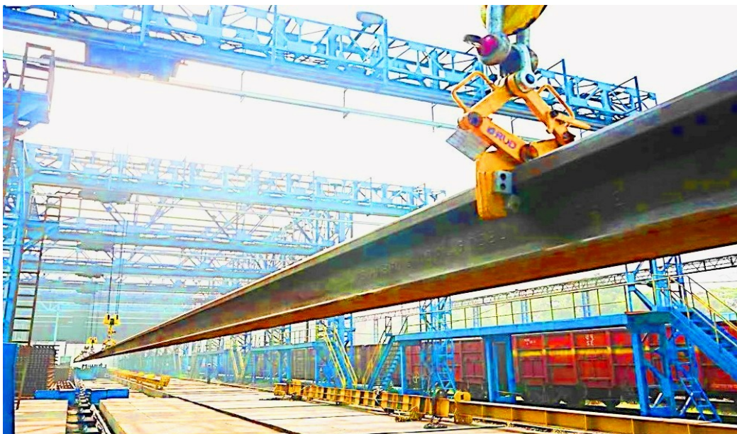
Synchronised Picking-Up of Long Rolled Rails, LRR, at Jindal Rail Manufacture Plant: source: JSPL
