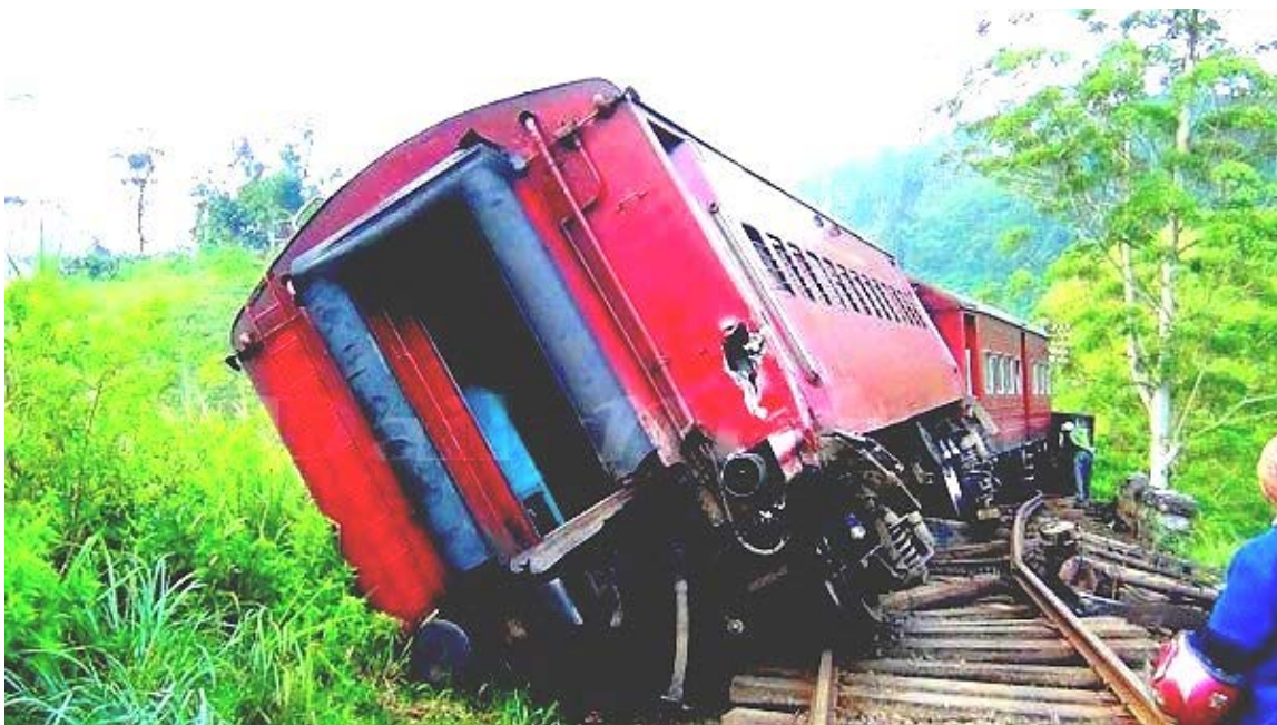
Fig. 2a: Train Derailments on Srilankan un-ballasted Rail-Tracks, especially on the Upcountry (Main) Line (Uva-Line) are frequent; Night Mail Derailment on un-ballasted Rail Track with Concrete Sleepers near Kotagala; Pict. by Daily Mirror
