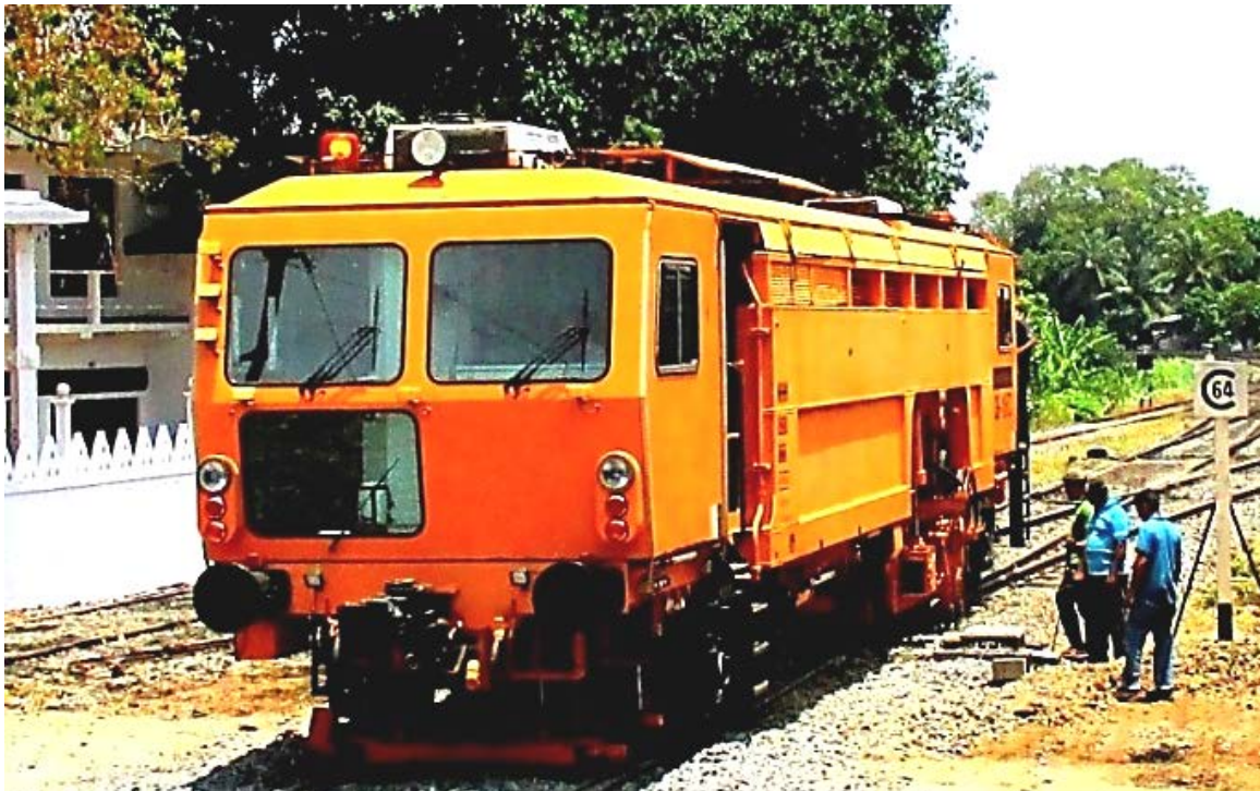
Fig. 21: New Sri Lanka Railway Plasser&Theurer on-Track Lifting, Aligning and Tamping Machine; Pict. by Primal Madusanka
