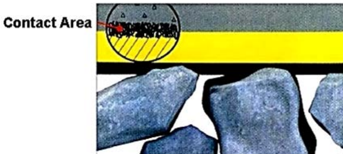
Fig. 4b: Increased Contact Area with Under-Sleeper Pads; Sketch by Getzner, Austria
