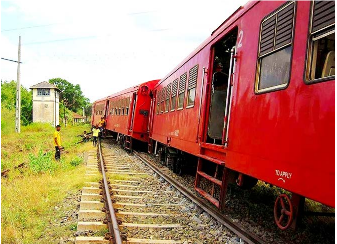
Fig. 2b: S11 Power-Set Derailment on poor ballasted Track of SLR Northern Line
