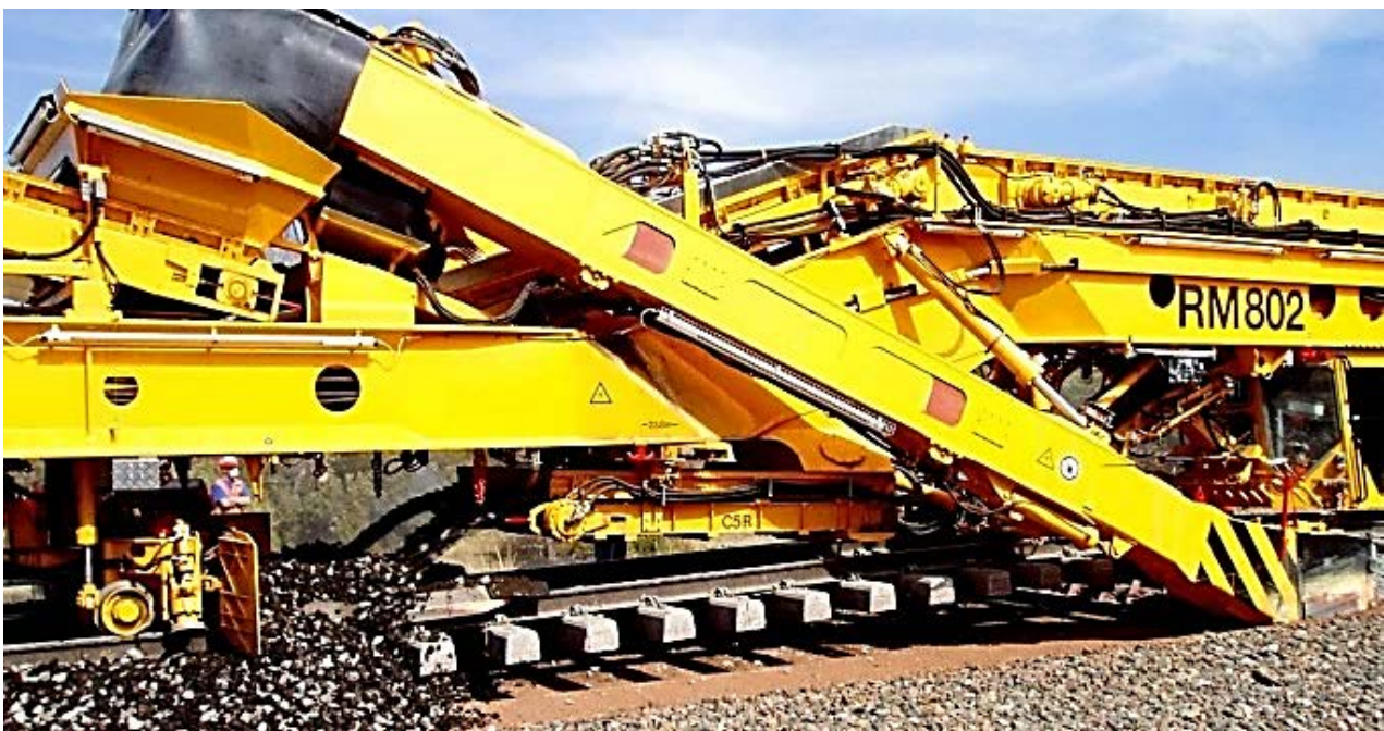
Fig. 13a: Plasser&Theurer Ballast Cleaning Machine, RM 802; Pict. by Plasser&Theurer
