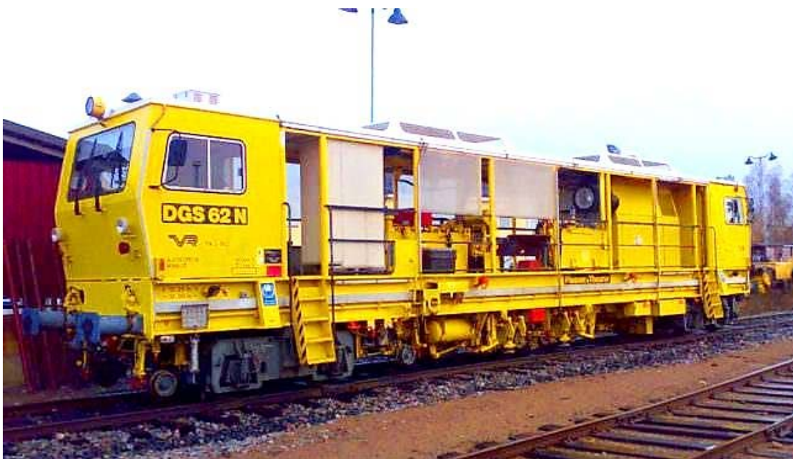
Fig. 23: Pl&Th Dynamic Track Stabilizer DGS 62 N; Pict. by Plasser&Theurer
