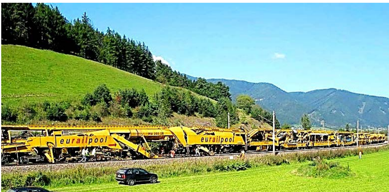
Fig. 13b: Plasser&Theurer PM 200 2R on-Track Rehabilitation Train; Pict by Plasser&Theurer
