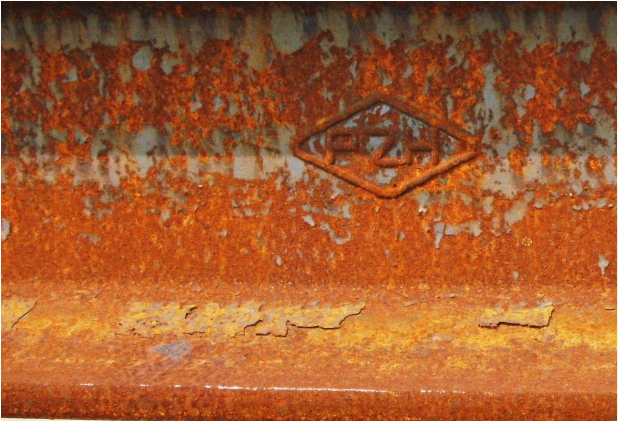
Corrosion on UIC60 E Rails, manufactured in China according to the European Standard EN 13674-1 by PZH Pangang Group, Pazhihua, Sichuan Province
