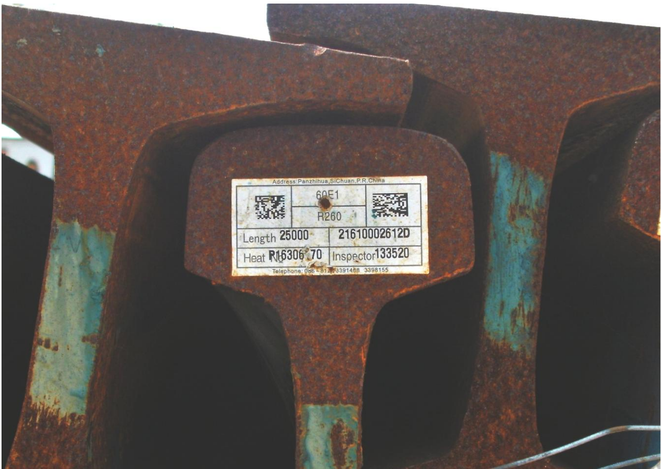
Corroded UIC60 E Rails for Matara-Beliatta Extension Project
