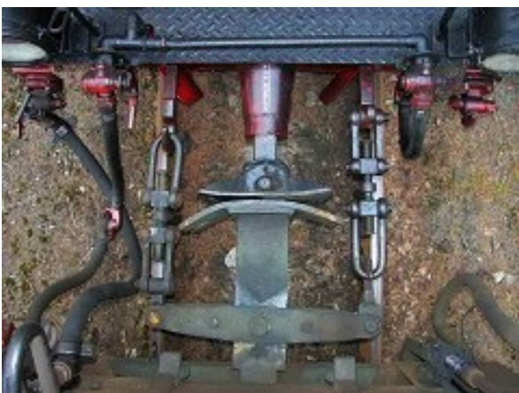
Jerk damping German Coupling Systems for NG Train-Sets with Telescope Damper
