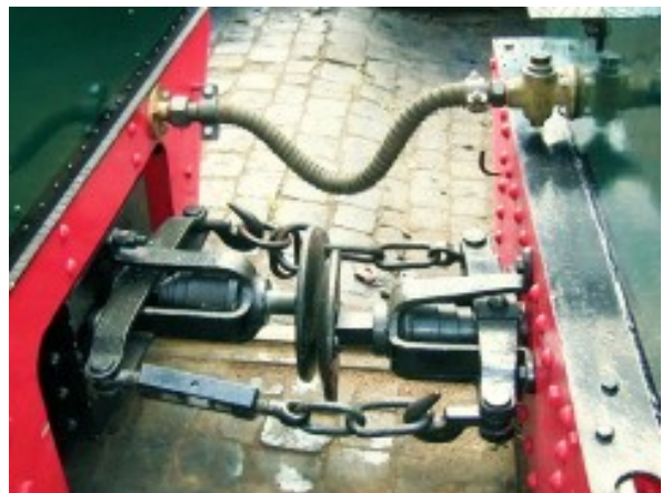
Jerk damping German Coupling Systems for NG Train-Sets with Telescope Damper
