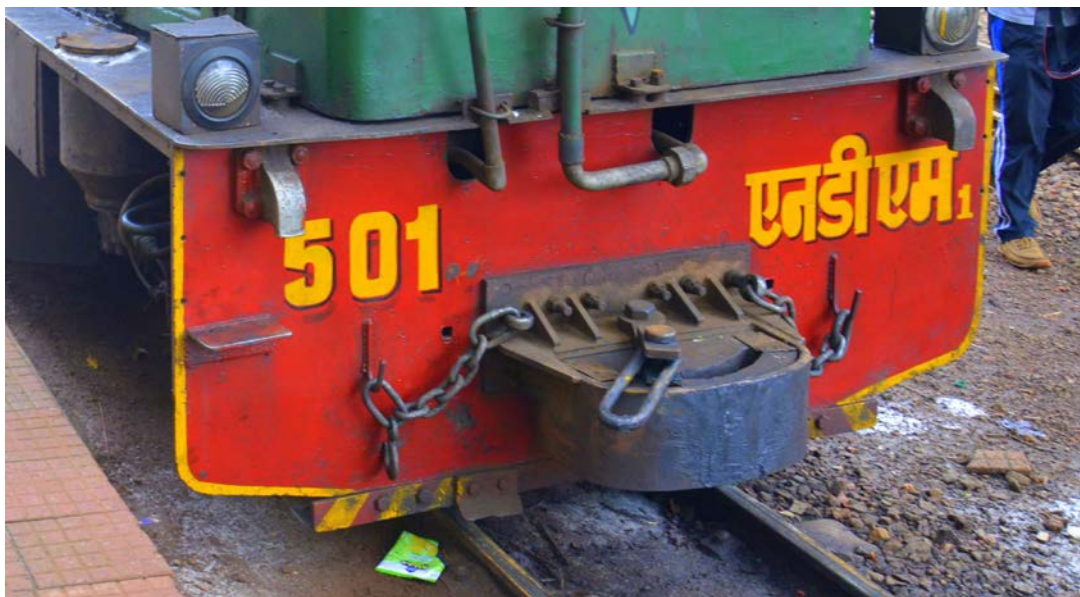
Inelastic simple Coupling Device
